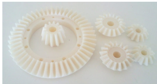
Fig. 4 - ABS Gears obtained by 3D Printing
