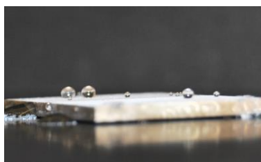
Figure 1 – water droplets lying over a Mg plate covered with two water-borne superhydrophobic top-coats
