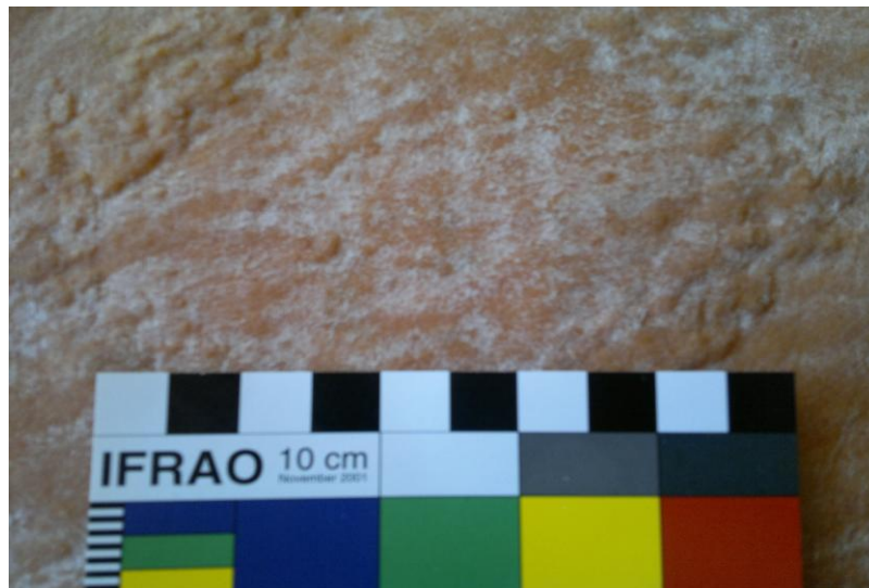
Figure 4: Talc engrained within the latex. G11, M-498. Source: ITM
