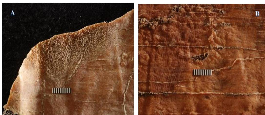
Figure 3: A: Fungi on the mold surface (AL-8 M-1122) B: Fungi between layers (AL-33 M-1133). Source: Silva 2011
