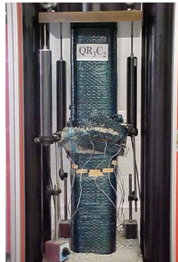
Figure 2 – Failure modes of CFRP confined columns
