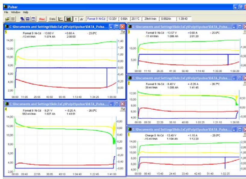
Fig. 2 The graphical interface of PCGraph program (the colors determine: blue – amperes, red – temperature, green – volts, yellow – dV/dt)
