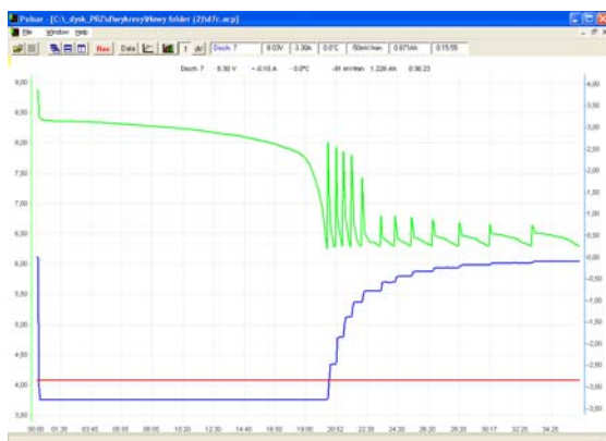
a) the characteristic of charging process in which after 22 minutes and 30 seconds there was a volt decrease. This situation means there is one weaker cell in the package
