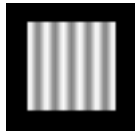
Fig.2 Measured object (simulation formula) O(x, y) = 1 + 0.3 \text{SIN}(kX)
