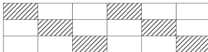
Fig. 5 Scheme of division of an interval of sampling on 6 parts, for definition of minimum correlation
