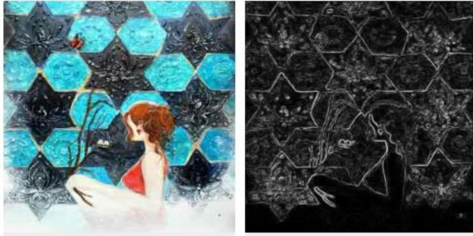
Figure 6: Sobel edge detection: original image and Sobel filtered image.
