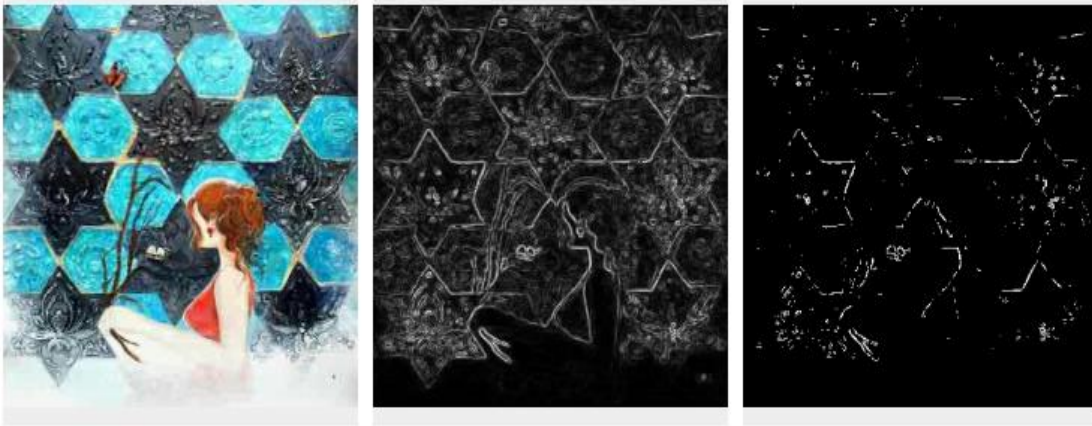
Figure 7: Sobel edge detection: original image, Sobel filtered (no threshold), and Sobel filtered (threshold of 0.5).
