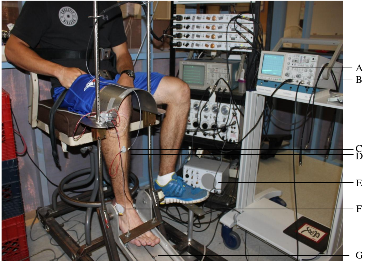
Figure 9. Experimental set up. Subjects were seated in the testing chair with real-time feedback of their force from the oscilloscope (A). A second oscilloscope (B) and a speaker (E) were used as real-time feedback for the experimenter to hone in on motor units. Surface, needle, and ground electrodes are shown as C, D, and F respectively. The load cell is located beneath the metal foot plate (G).
