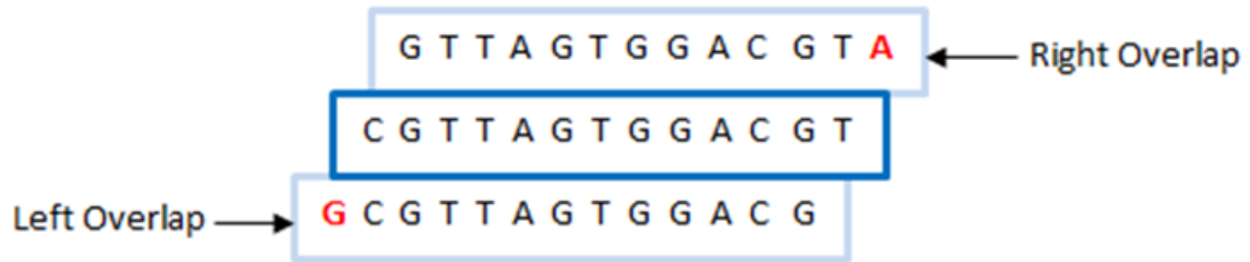
Figure 3.2: For a read of length n , the right overlap (postfix) is a read for which its base-pairs positions 1 to n - 1 are matched to the original read's base-pairs from positions 2 to n . Also, its left overlap (prefix) is a read for which its base-pairs from positions 2 to n are matched to the original read's base-pairs from positions 1 to n - 1 .
