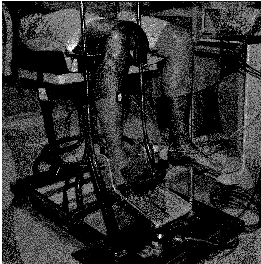
Figure 11. Subject test position and experimental set-up. The load cell was at the bottom of the foot-plate. There were separate belts for the thighs and waist to secure the legs and hips, respectively.
