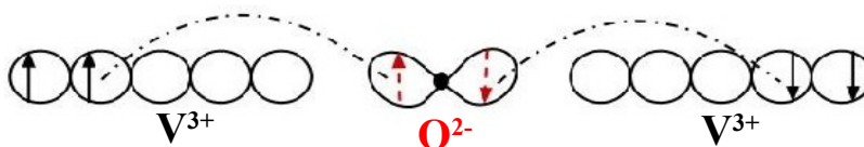
Figure 2.5 Geometry of the indirect interaction in \text{RVO}_3 metal-oxide along V-O-V bonds, adopted from Ref. [2].
