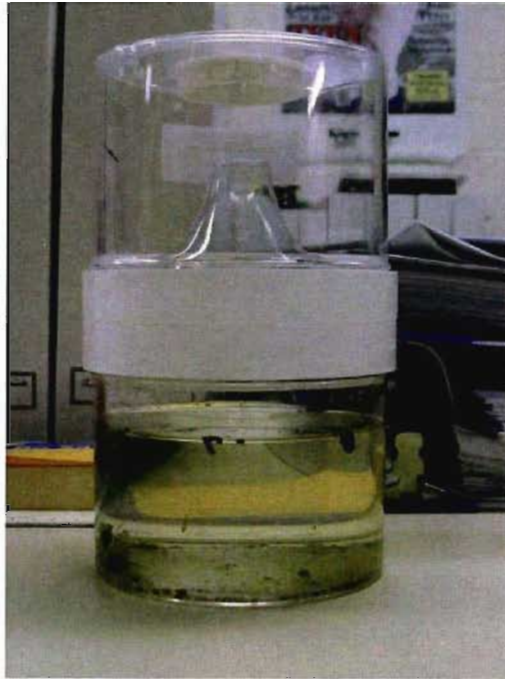
Figure 2.14. Mosquito breeders used to rear Anopheles larvae and adults. Larvae and pupae develop in the water in the lower chamber and adults fly up through a funnel-shaped barrier to rest and feed in the upper chamber.
