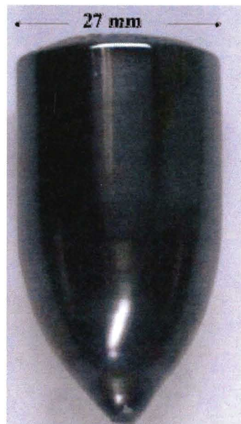
Figure 1.14: Verneuil grown Strontium Titanate boule [29].
