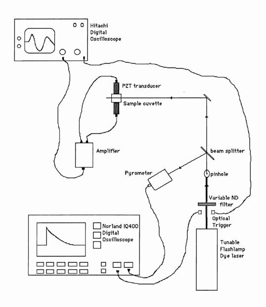
In order to increase the signal-to-noise ratio a combination of two PZT transducers attached to the opposite walls of the cuvette was used (Figure 5). If the laser beam passes exactly through the middle of the cuvette the signals from the two detectors will be in phase and can be superimposed (Nitsch et al., 1988).
