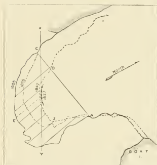
FIG. 4.—Outlines of Horseshoe Fall in 1842, 1875, and 1905, with lines used in computing the rate of recession. The line of crosses suggests a position of part of the crest in 1827.
