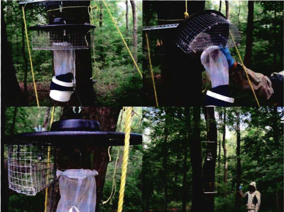
Figure 1. Photographs of a modified CDC miniature light trap ( \text{CO}_2 and light removed) with a small wire cage used to hold either a guinea pig or chicken as a host attractant.
