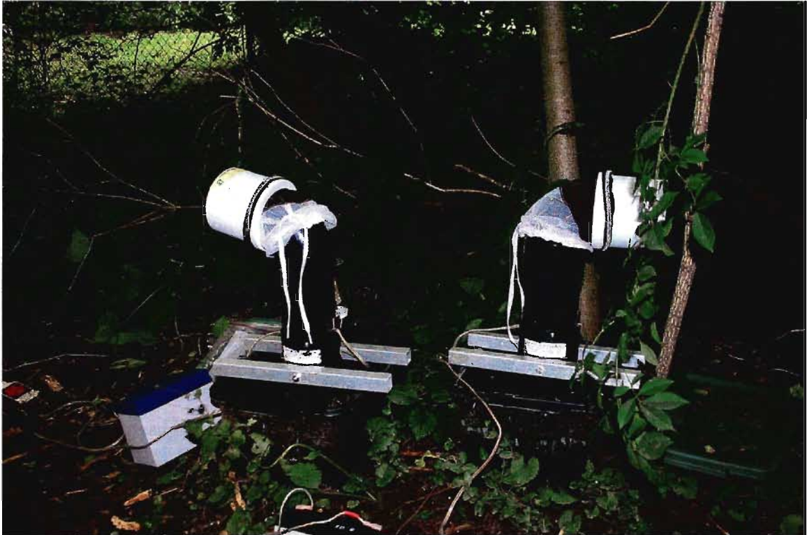
Figure 2. Photograph of modified CDC gravid traps used to capture mosquitoes for blood meal identification. To modify the traps a 90° PVC elbow was added to the top of the chimney and a CDC light trap (Model 512, John W. Hock Co., Gainesville, FL) sock was used to hold the captured mosquitoes. This modification allowed for easier removal of the mosquitoes, and caused less damage to the mosquitoes.
