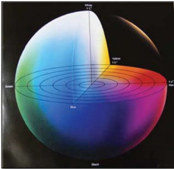
Figure 1: Colour coordinates in the L*a*b* scale (CIE 1976).
