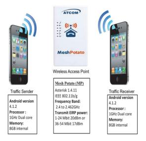
Figure 3: Wireless testbed network setup.
