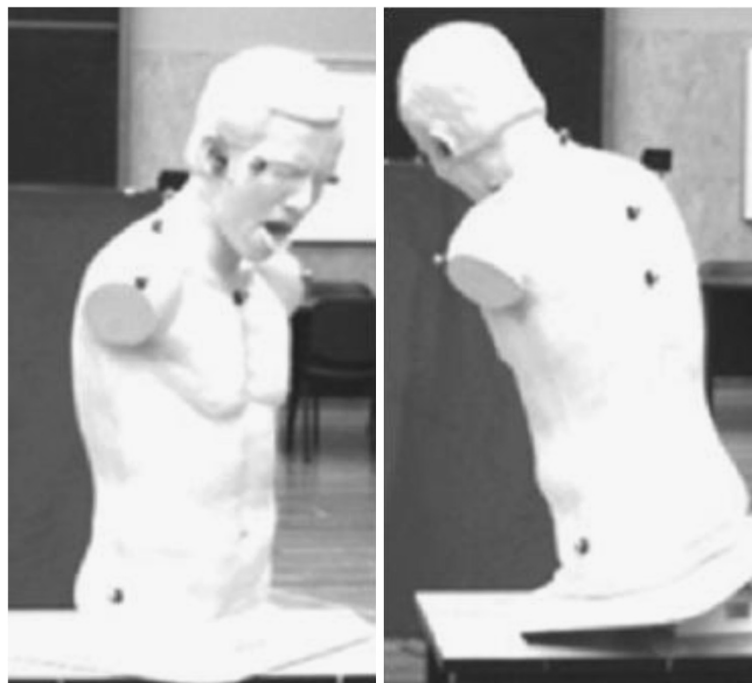
Figure 1 The placement of the reflective markers on the mannequin.
