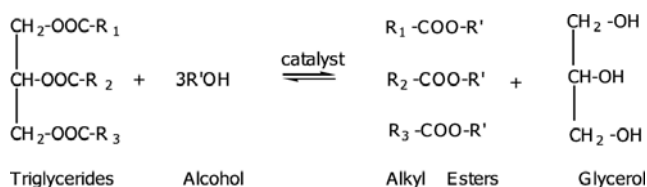
Fig. 1 Transesterification of triglyceride with alkyl alcohol
