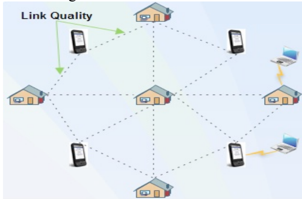
Fig. 1: A dynamic mesh network, applicable to a rural area, with static nodes inside homes, and mobile nodes on cell phones. Note that link quality in such networks is continually changing as phones move around.
