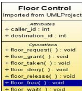
Fig. 4. Floor control methods illustrate the high level design of the floor control of the PoC application. The methods manage the PoC application's functional operation to give a user the ability to speak in half-duplex mode.
