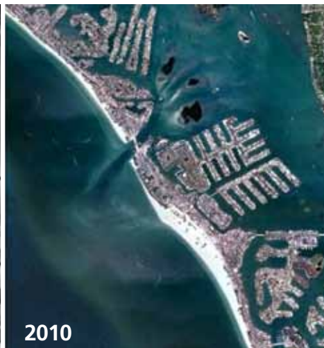
1950s–1960s Finger channels were constructed over mangrove and oyster reef habitats in South Florida. The reduction in bay size from filling also had a substantial impact on the tidal inlets and on sediment supply to adjacent beaches. Photos: Courtesy of Ping Wang
