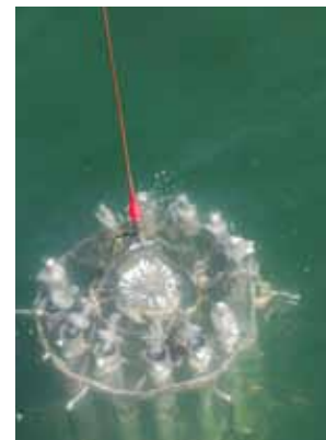
A CTD (conductivity, temperature, depth) device detects how the conductivity and temperature of the water column change relative to depth. Photo: NOAA
