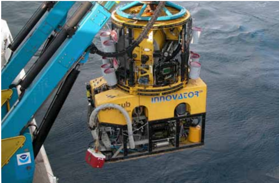
A remotely operated vehicle is used to collect samples from the ocean floor. Photo: Gulf of Mexico Deep Sea Habitats Expedition/NOAA/OAR/OER
