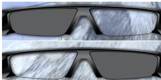
Figure 5.5: Active Stereo - shutter glasses behaviour
