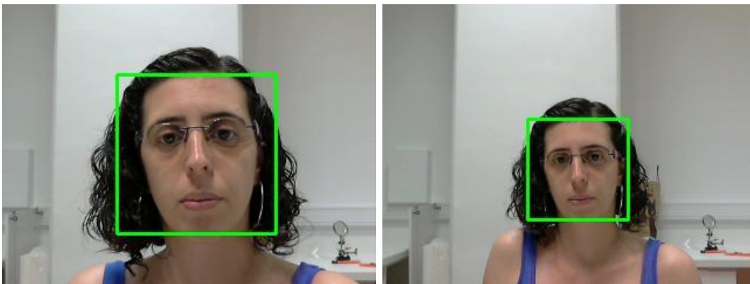
Figure 3.18 Face detection with the user away from the screen 50cm on left and 100cm right
