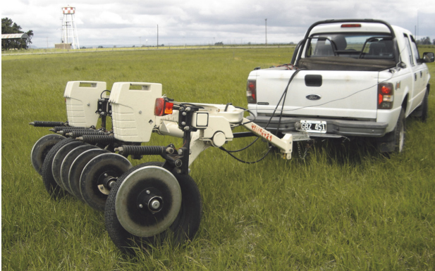
Figure 2. The Veris 3100 System mounted behind the truck.
