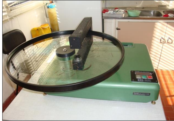
Figure 5. Measurements of fine roots using Comair Root Length equipment.
