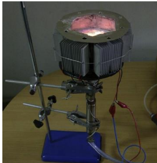
Figure 8. The micro cogeneration system developed by Ismail et al. (2013).
