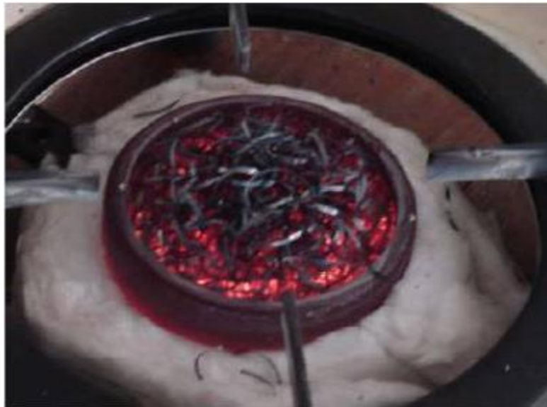
Figure 5. One of the porous burners studied by Pantangi et al. (2007).
