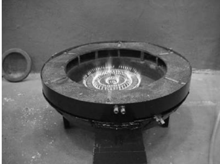
Figure 3. The porous radiant recirculating burner developed by Jugjai and Rungsimuntuchart (2002).
