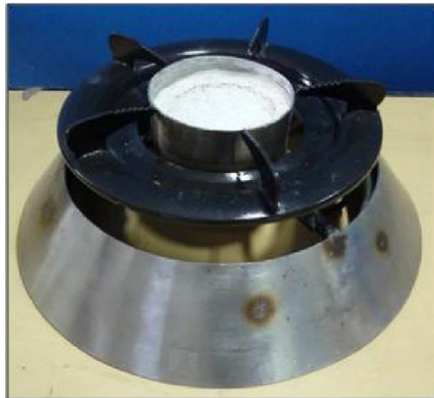
Figure 7. The surface stabilized burner developed by Mujeebu et al. (2011c).
