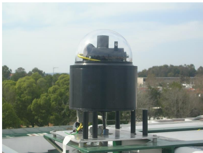
Figure 4.5- The MIGE platform installed on the roof of the container where the SPATRAM instrument is placed. This platform ensure the possibility to carry out measurements in off-axis configuration along many azimuthally directions since the horizon line is almost completely free (from Domingues, 2011).
