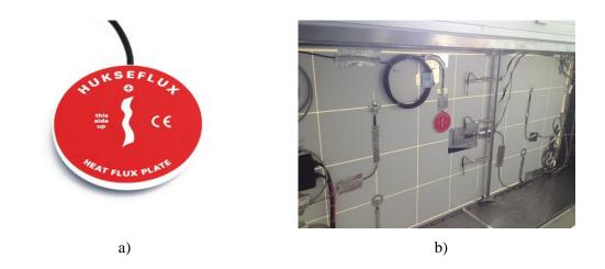
Fig. 5.9. Hukseflux HFP01 fluxmeter (a). Hukseflux HFP01 fluxmeter installed at PV interior layer (b)
