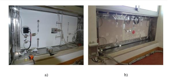
Fig. 5.4. Sensors installed on inner PV layer (a), Sensors installed on inner PCM layer (b)
