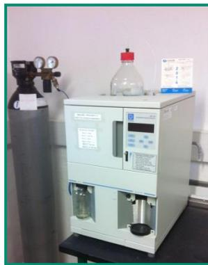
**Figura 14** - “Accelerated Solvent Extractor”
