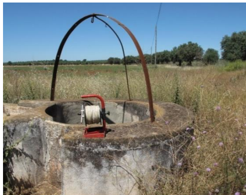
Figure 15: Example of a dug well where SWL was measured resorting to a piezometric probe as illustrated in the image.
