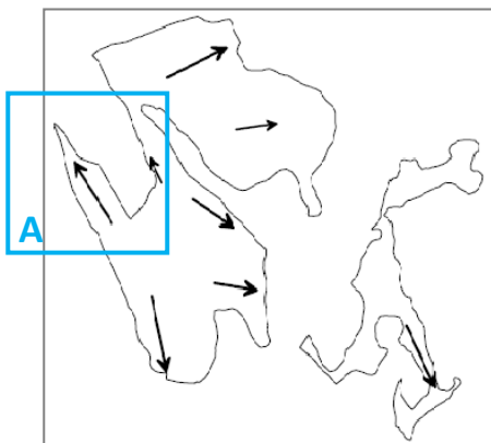
Figure 14: Water flow directions in the Aquifer System of Elvas-Vila Boim; A – Area covered by the study area (Adapted from ERHSA 2001).
