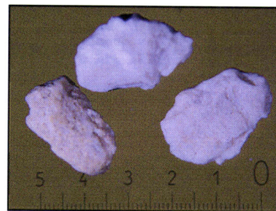
Figure 1.7. Aspect of sepiolite grains.
