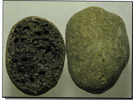
Figure B-1. Typical aspect of LECA grains.
