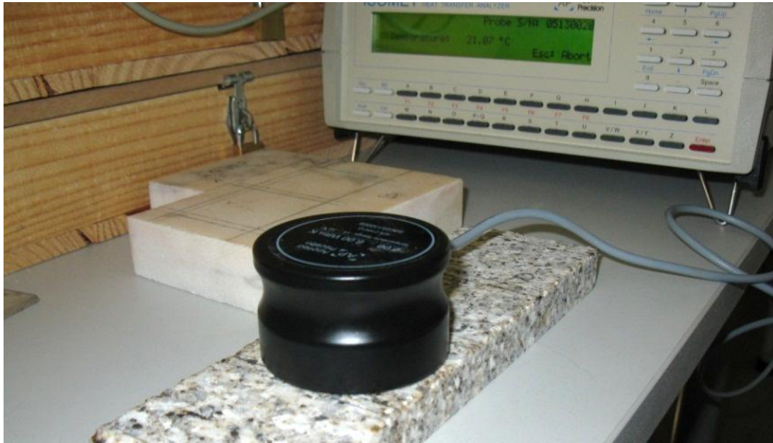
Fig. 4 – Heat Transfer Analyser ISOMET 2104. The measuring probe is the black device on top of the rock sample.
