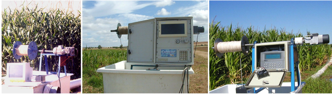
Figure 2. Evolution of the automatic controller. Left : the first version using an inverter to control the motor and the movement of the pulg. Centre : second version using a modified PC to directly control the motor. Right : final version using a microcontroller to fully operate the irrigation system. This figure is available in colour online at wileyonlinelibrary.com/journal/ird
