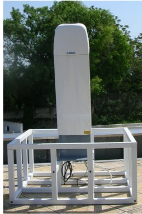
Fig. 1. VAISALA Ceilometer CL31, installed in the CGE observatory in Évora (38°34' N, 7°54' W, 300m a.m.s.l.), in the South of Portugal.
