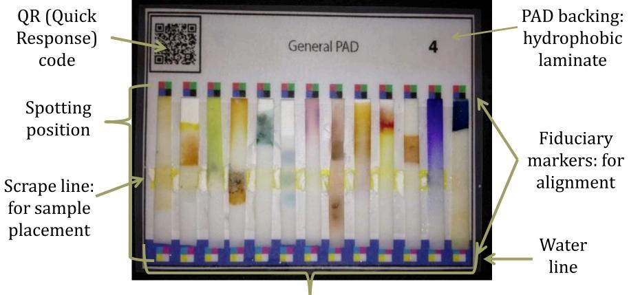
Lanes for different colorimetric tests: hydrophilic lanes of paper
