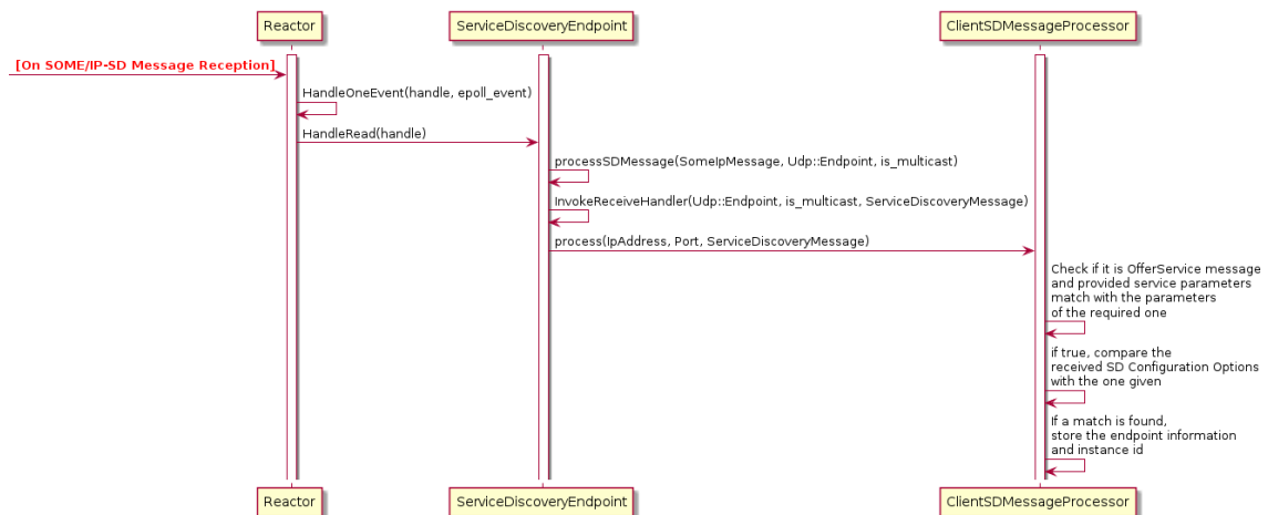
Figure 5.5: SOME/IP-SD Message Reception on Client
