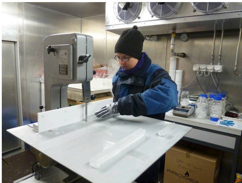
Fig. 5.1 Ice core cutting in the cold room at PSI.
