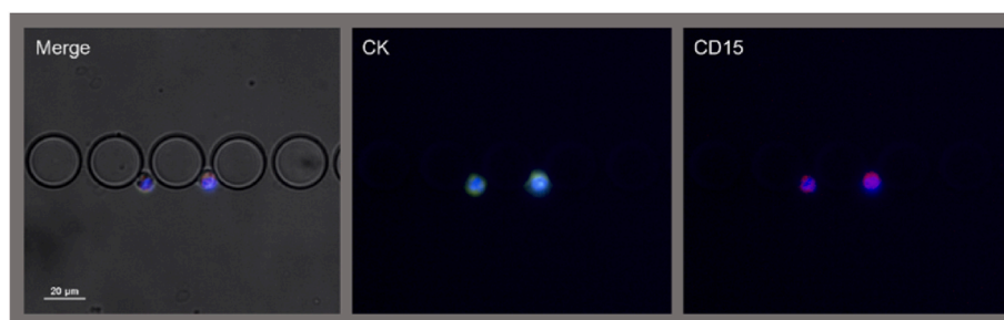
Fig. 4. Healthy whole blood sample processed on the RUBYchip™ and directly labelled by immunocytochemistry against a pan-CK (green), CD15 (red) antibodies and DAPI (blue). All images are at the same magnification. (For interpretation of the references to color in this figure legend, the reader is referred to the Web version of this article.)
