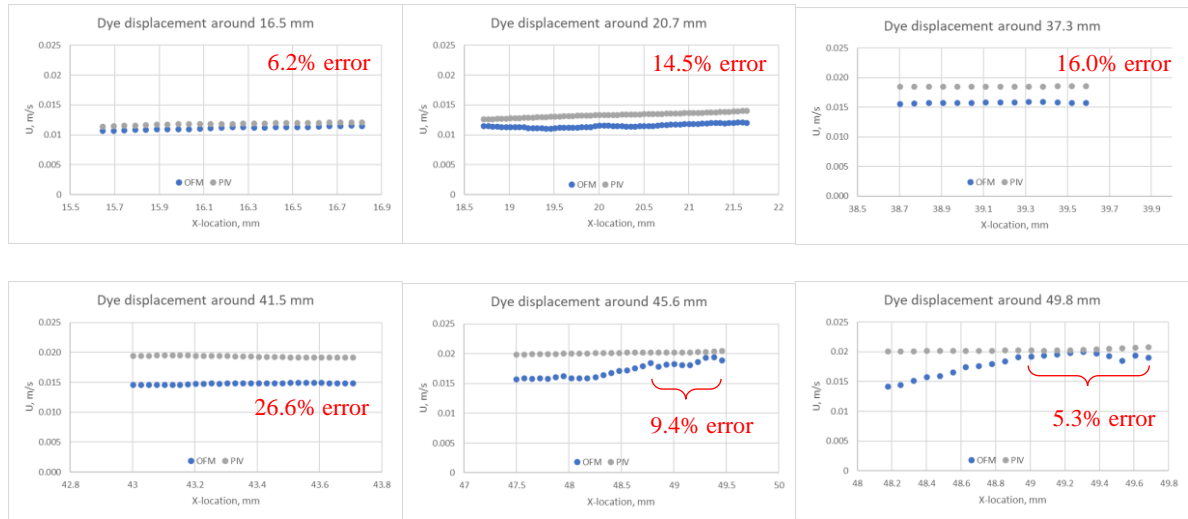
Figure 42: Velocity comparison between OFM technique and PIV technique for various dye displacement positions.
