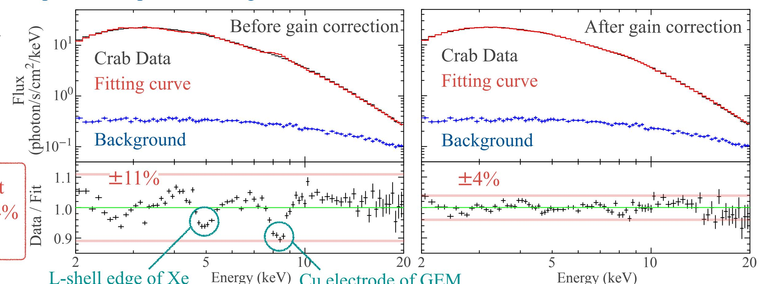
The ratio of the data to the fit curve improved from 11% to 4% in the range of 2–10 keV.
