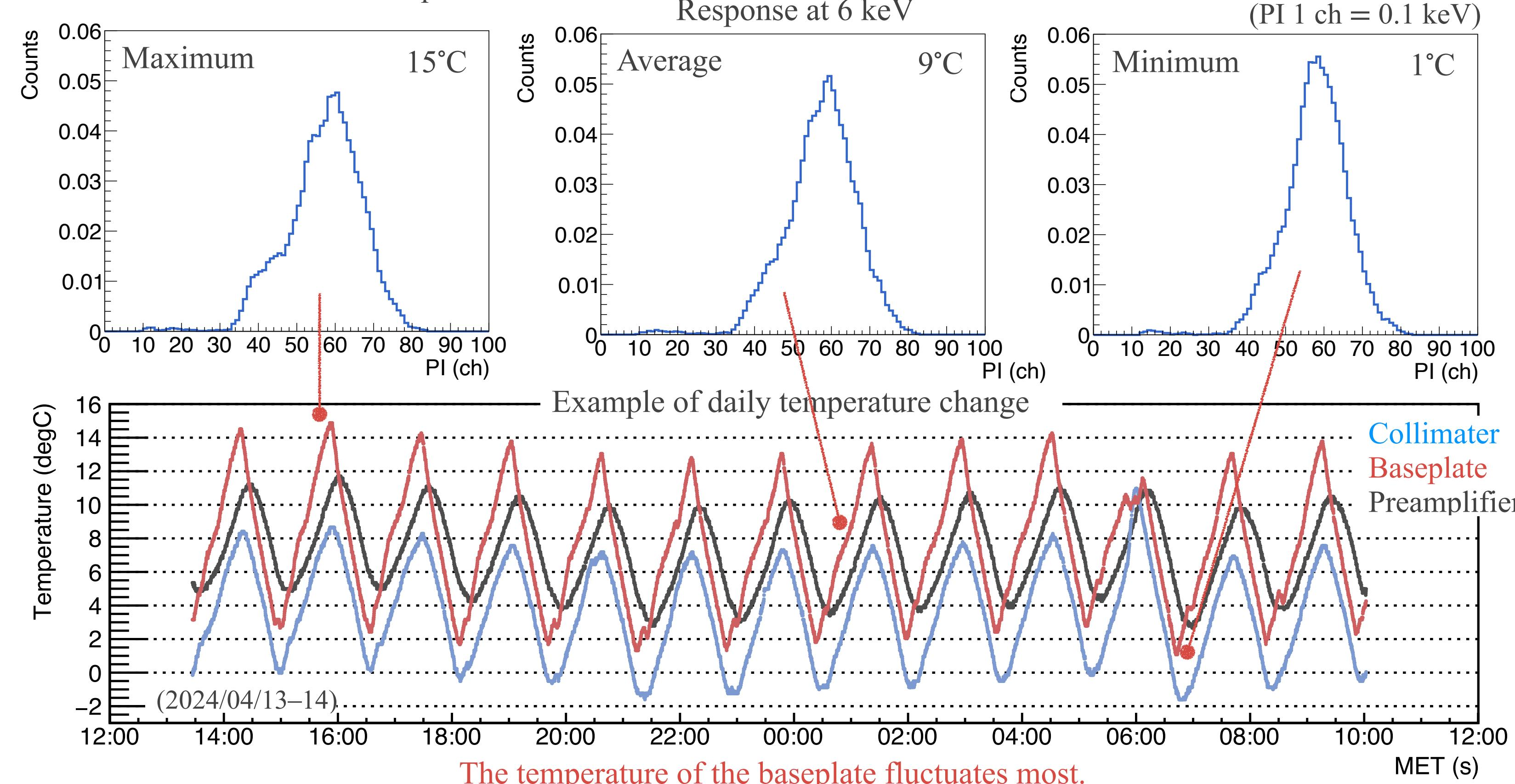
The temperature of the baseplate fluctuates most.
