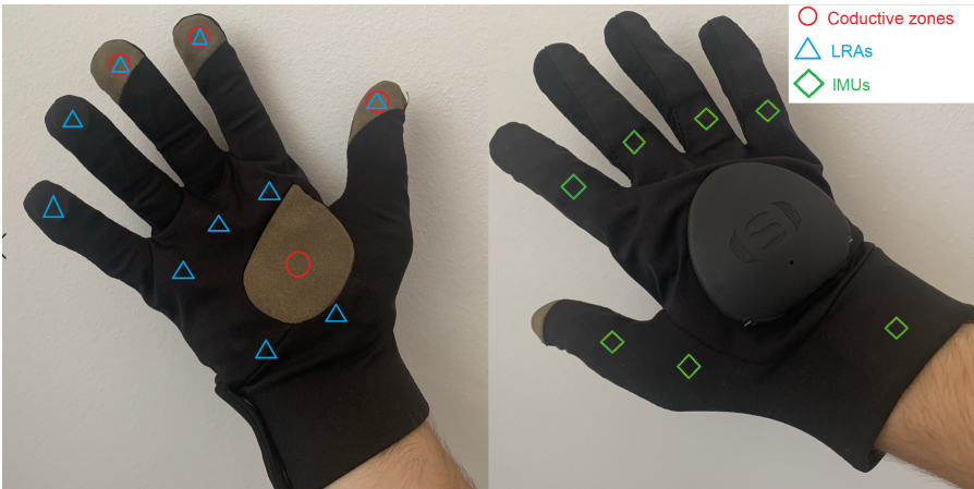
Figure 15.2 Sensors and actuators of Sensorial XR [16].
