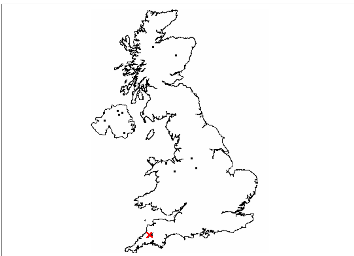
Figure 1.2 Example of a subject site (red cross) and the most hydrologically similar gauged catchments (black squares) included in the FEH pooling-group.
