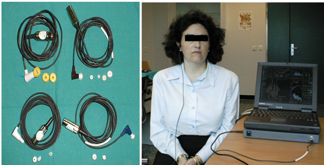
Figure 23. TEOAE software “ILO 292”; Contents: Ear probe, Small speaker, Microphon and Response Analyzer connected to computer (Our photo)
