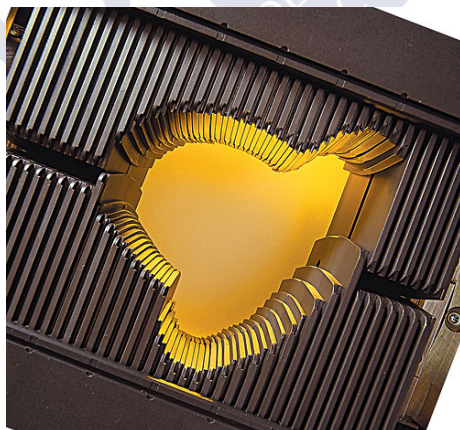
FIGURE 1.4: Multileaf collimator made of several independently moving opposed leaf pairs made of tungsten, typically projecting a 1 cm shadow at the isocenter.
