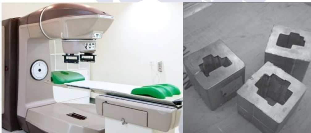
FIGURE 1.3: Left: Theratron 780 ^{60}\text{Co} radiotherapy unit. Right: cerrobend blocks prepared from the beam eye view of the tumor of an specific patient
