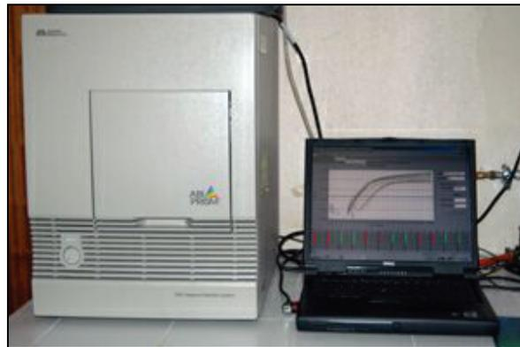
**Figura 8.** PCR Cuantitativo ABI PRISM 7000 Sequence Detection System. Applied Biosystems.
