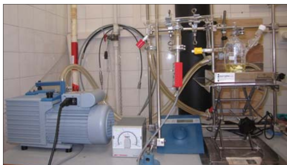
Fig.A.1. Picture and scheme of the vacuum line. (E1) Glass line, (E2) vacuum pump, (E3) sample flask, (E4) magnetic stirrer, (V1, V2, V3) valves, (I1) vacuummeter.
