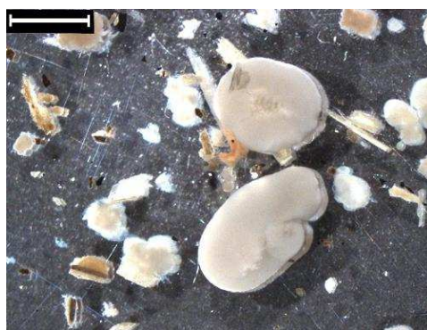
Figure 7.4. Picture of the AGS fed to the anaerobic digester in Stage IC. The size bar corresponds to 2 mm.
